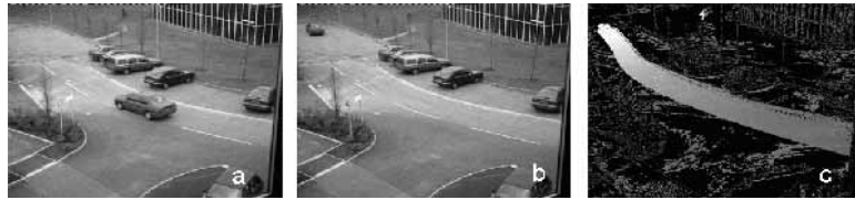
Fig. 1. Permanency effect: (a) one image of a sequence, (b) same perspective after some seconds, (c) motion trails as represented on the permanence memory
