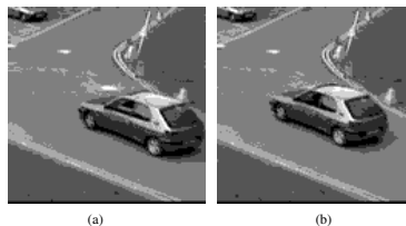
Fig. 5. Image segmented into 8 gray level bands (a) at t = 0 , (b) at t = 15 , with a frame rate of \Delta t = 0.04 seconds
