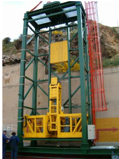
Figure 4-1. Primary Positioning System with both arm joint (yellow) and joint on tracks (green) of the EFTCoR
