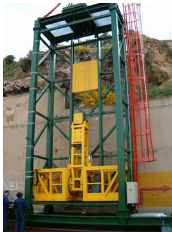
Figure 7-30. Primary Positioning System with both arm joint (yellow) and joint on tracks (green) of the EFTCoR system
