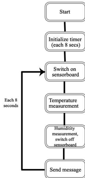
Figure 1. IntellBuildApp operation
