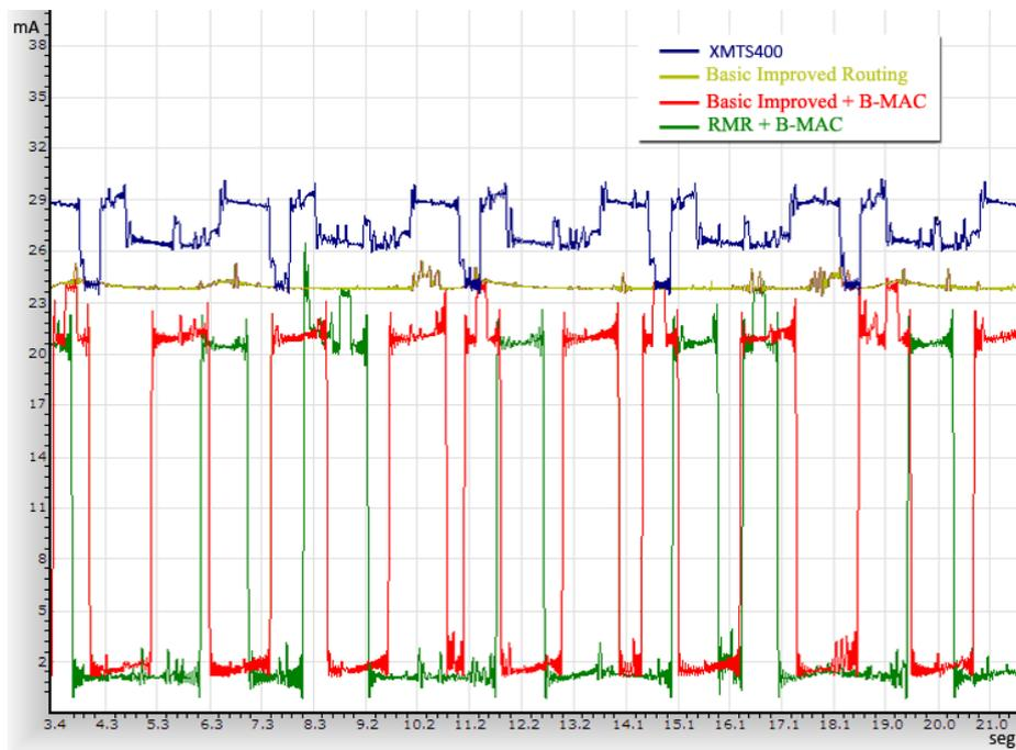
Figure 4. Instantaneous power consumption (node 2)
