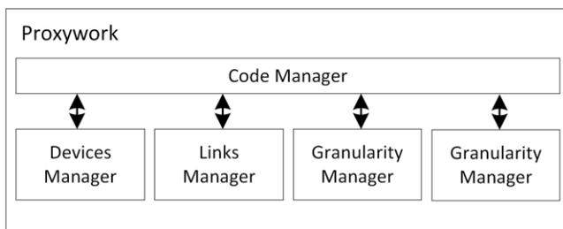
Figure 3 Proxywork software architecture
