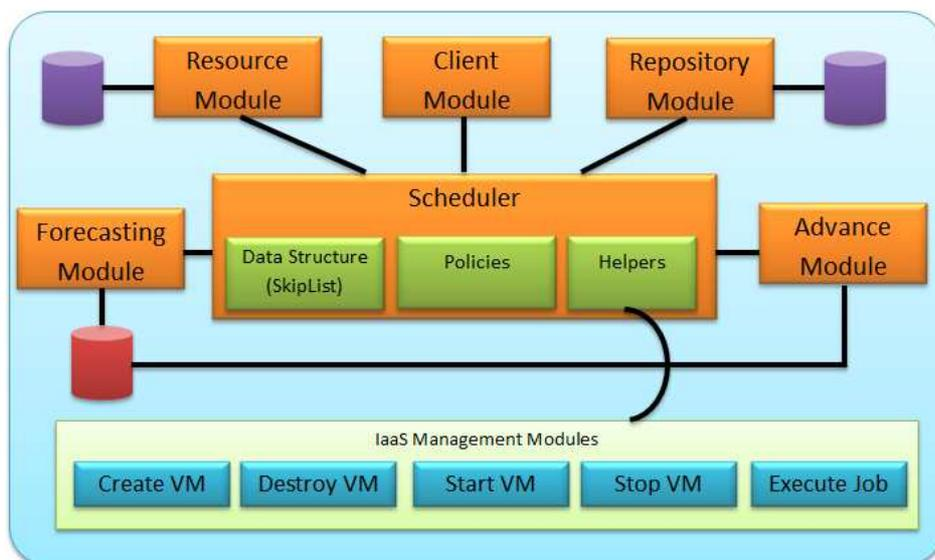
Figura 2: Nacreous internal architecture.
