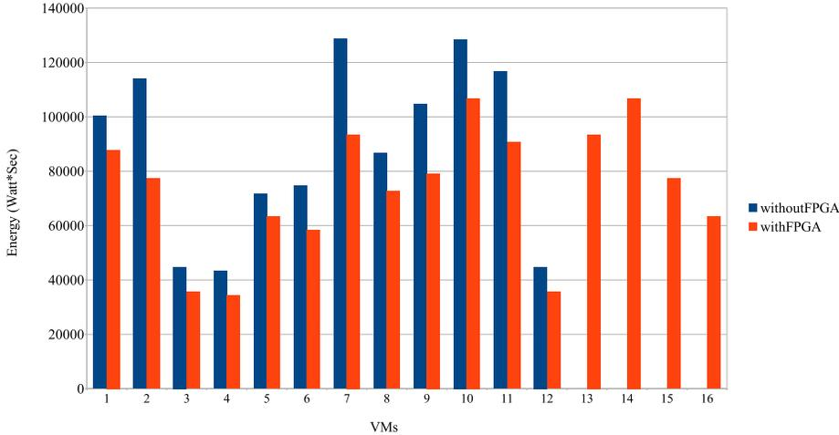
Figure 2: Number of video VMs processed and Energy per VM for FPGA and non-FPGA configurations
