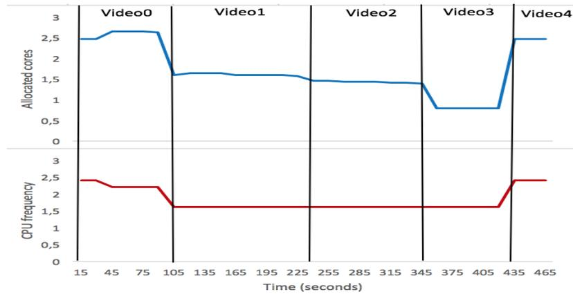
(a) Core and CPU frequency allocations by the optimizer for a video running on server CPUs.
