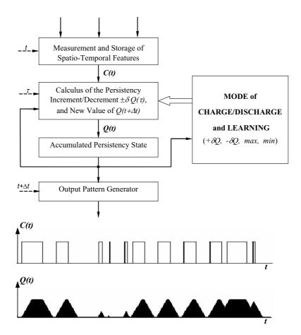
**Fig. 3.** The AC working memory model (upper part) and an example of the temporal evolution of the accumulated persistency state, Q(t), in response to an specific sequence of values of a detected feature, C(t), (lower part)
