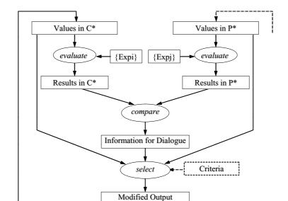
Fig. 2. Recurrent ALI inferential scheme. The results of the evaluation in the central  $(C^*)$  and peripheral  $(P^*)$  parts of the feedback receptive field are first compared and the result of this comparison is used to select the updated output.
